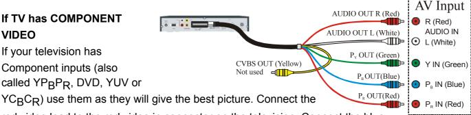
red video lead to the red video in connector on the television. Connect the blue to the blue and the green to the green.
